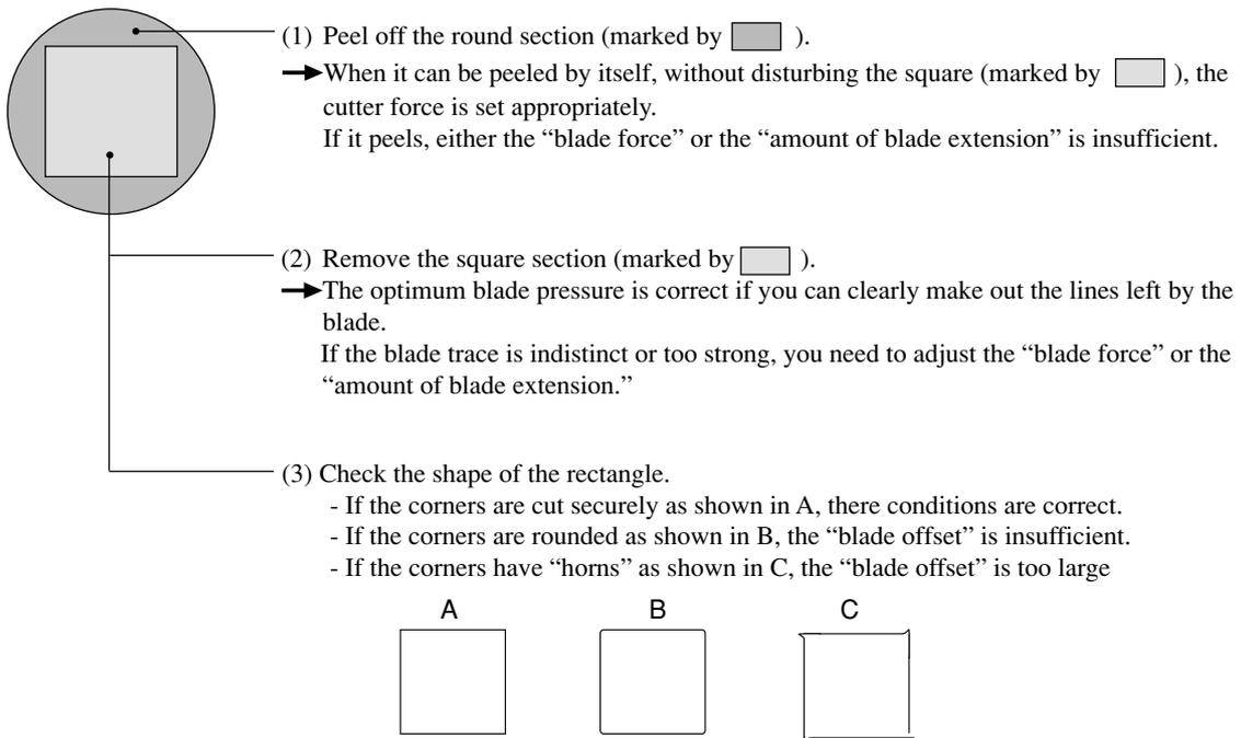
If the test cutting shows problems with the material cutting results, adjust the cutting conditions.
