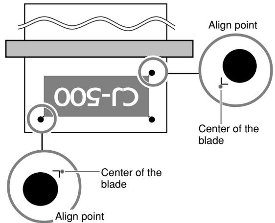
Align the center of the blade with the base point or the align point.
