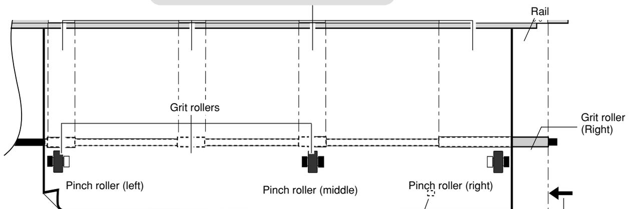
\* Position the left and right pinch rollers over the material, near the edges.
