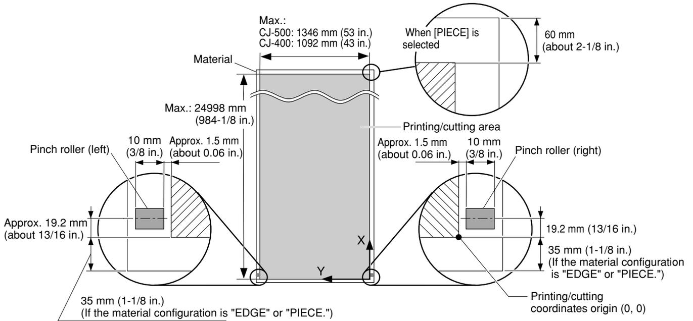
\* The arrows in the figure indicating the X and Y directions indicate respectively the positive directions of the X axis and Y axis.
