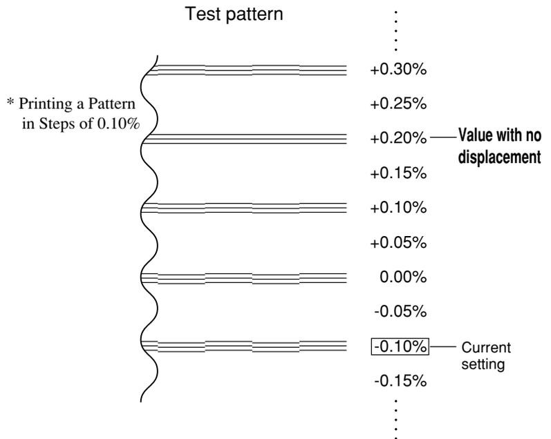
**5** Check the test pattern and choose a value with no displacement.
