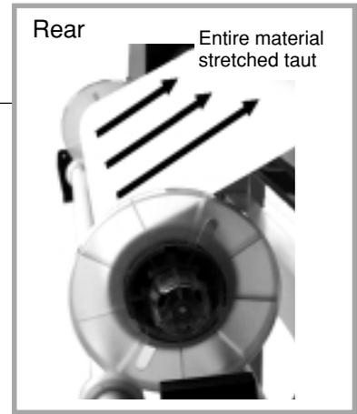
\* If there is slackness in the loaded material, the material may move at an angle and come loose from the pinch rollers.
