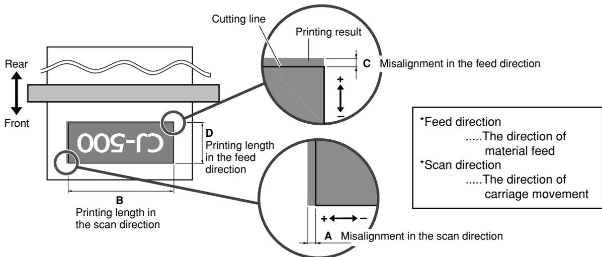
**2** Calculate the percentage of cutting-length displacement relative to the printing length.
