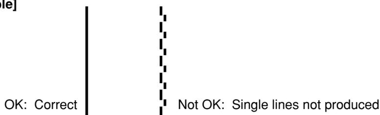
If misalignment like in the example occurs when the printing direction for [PRINT QUALITY] has been set to [BI-DIRECTION] (bidirectional), then carry out correction at the [BIDIRECTION] menu (see "User's Reference -- Making Corrections for Printing -- Bidirectional Correction").
