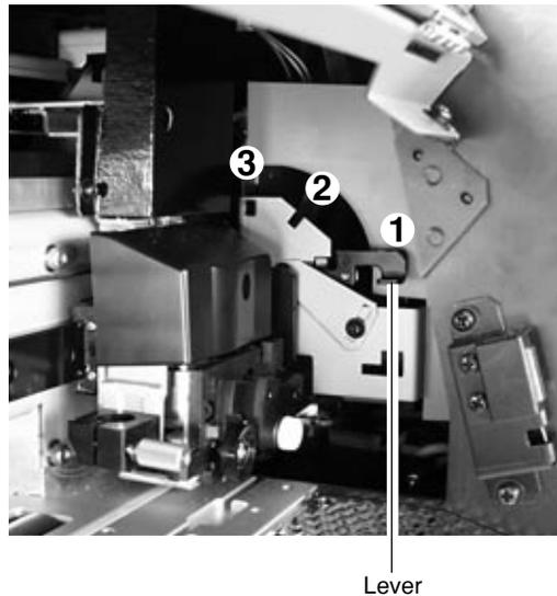
\* Be sure that the carriage is in standby position before attempting to move the lever.
