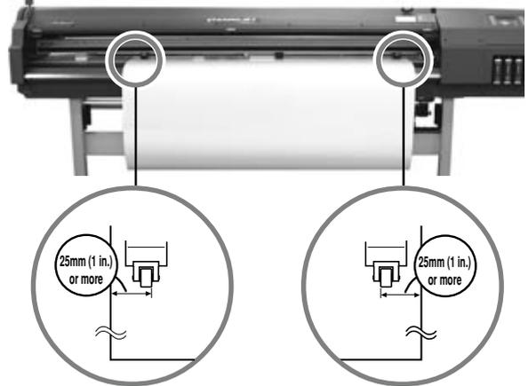
\*Make sure the pinch rollers are positioned above the grit rollers.
