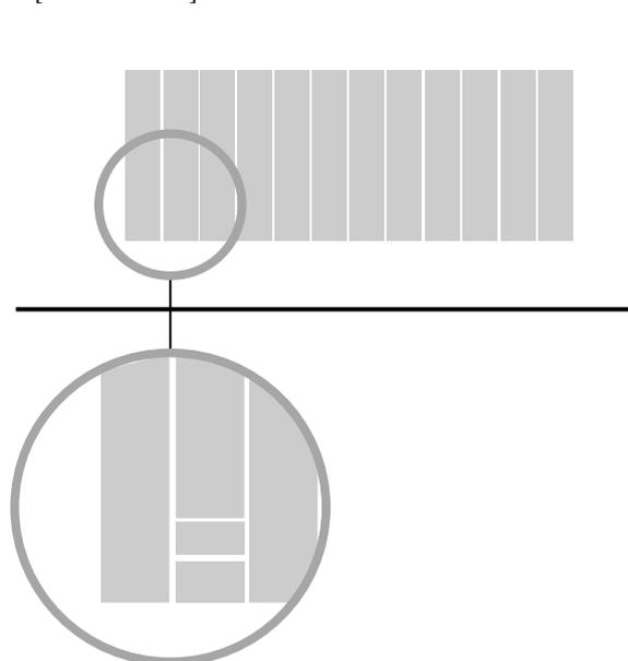
If there are any missing dots or other evidence of a drop in printing quality, clean the head (see "Maintenance -- Cleaning the Printing Heads").
