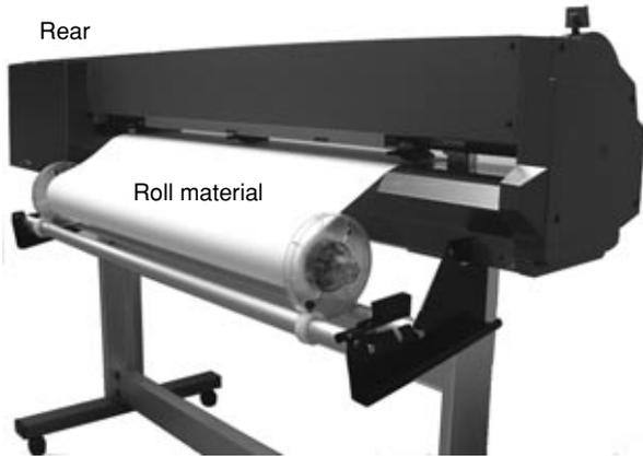
\*Use material that is wider by 50 mm (2 in.) or more than the width of the printing or cutting to be performed.
