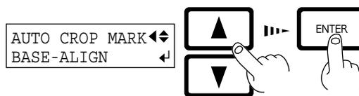
**BASE-ALIGN** : Aligns the start position for output and the axis slant and length.
