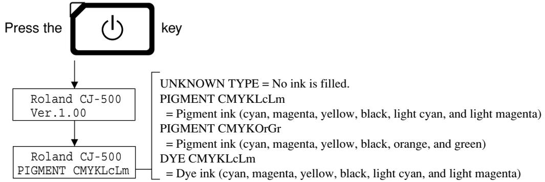
With pigment inks, do not insert ink cartridges for orange or green when using light cyan and light magenta. Also, do not insert the ink cartridges for light cyan or light magenta when using orange and green.
