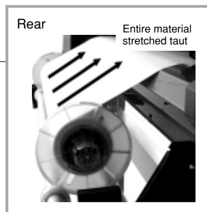
\* If there is slackness in the loaded material, the material may move at an angle and come loose from the pinch rollers.
