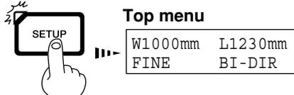
If a pinch roller is positioned over an area where is no grit roller, the message shown at below appears when you press the [SETUP] key.
