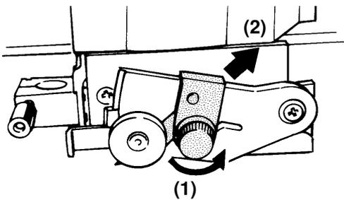
If the blade remains in the carriage, use commercially available tweezers to remove it.
